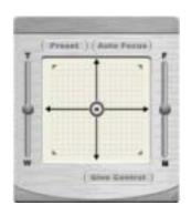
**Auto-Focus:** The VersaCam IC-360 has an auto-focus function. However, you can control and optimize the focus of the image manually by dragging the ball on the right vertical bar 'F'-'N' (farther, nearer) on the control panel.
